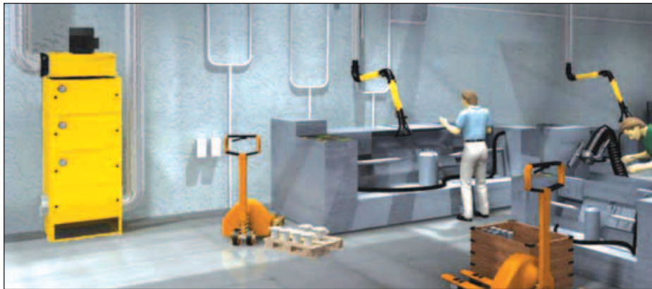
Source extractions arm system connected to MistEliminator
