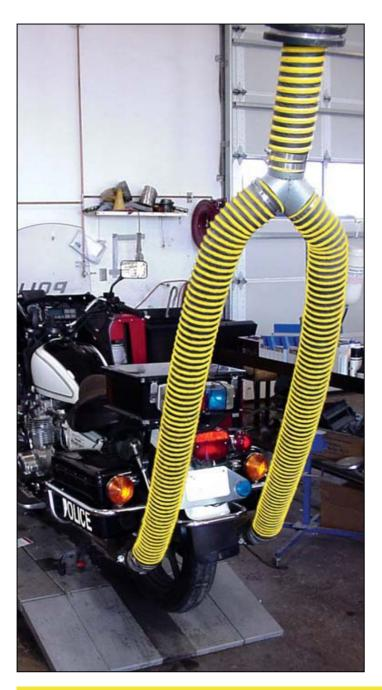
PlymoVent has reintroduced the YS adapter. The YS adapter is made from crush resistant hose that will stand up to the day-to-day abuse of high volume workshops.
